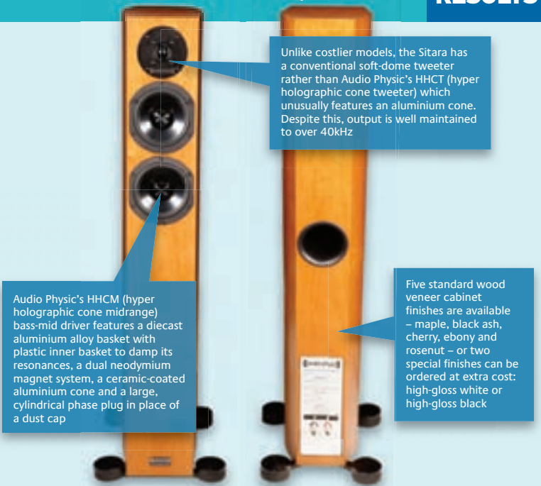
ABOVE: Audio Physic's bass-mid driver has a ceramic-coated aluminium cone with large cylindrical phase plug
