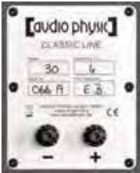
The terminal lists some of the loudspeaker's technical details and features "next-gen" cable connectors made by WBT.
