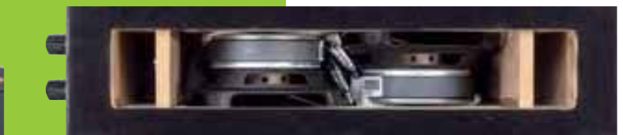
The image on the left shows the woofer unit, which is closed at the top, when removed from the loudspeaker cabinet. The woofers are positioned next to each other in the compact unit and are covered by the base panel of the loudspeaker when installed in the cabinet. Removing this base panel provides an insight into the woofers' direct sound outlet and the reflex ports on both sides (as shown below).
